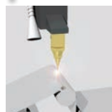
Collecting fumes generated during laser cutting.
